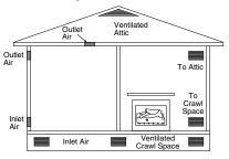
Figure 3 - Ventilation Air from Outdoors
